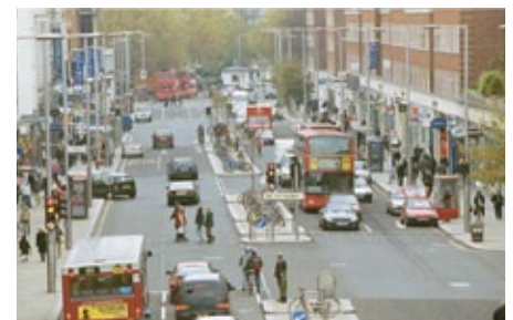
High Street Kensington, where crossings have been made more direct and a median strip accommodates cycle parking and tree planting.
