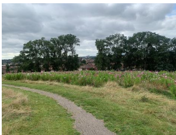
Walking path is not DDA compliant (1.5m wide is the standard required)
