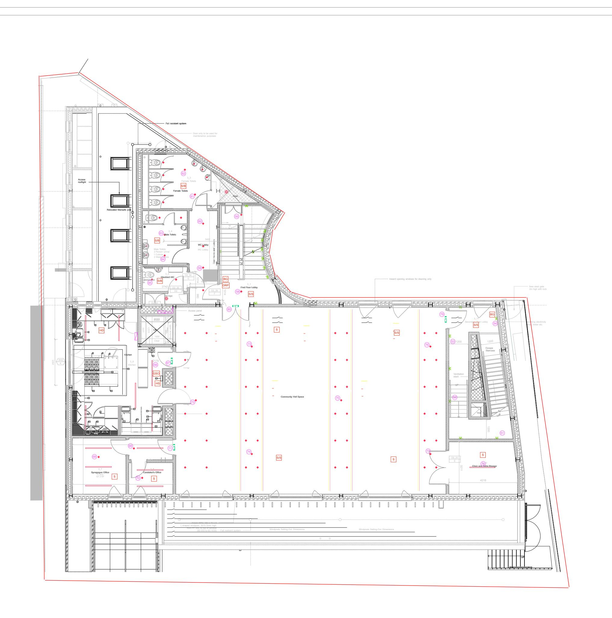
(01) EMERGENCY LIGHT FITTING Exit EMERGENCY EXIT / RUNNING MAN BG FIRE ALARM/ BREAK GLASS S SMOKE DETECTOR S/S SMOKE DETECTOR WITH SOUNDER SMOKE DETECTOR WITH STROBE LIGHT FP FIRE PANEL DRP DISABLED REFUGE POINT HD HEAT DETECTOR HS HEAT DETECTOR WITH SOUNDER FE FIRE EXTIGUISHER EL EXTERNAL EMERGENCY STROBE LIGHT ESO ELEVATION SHUT OFF GSO GAS SHUT OFF
