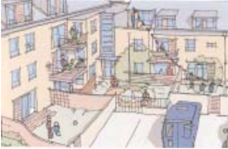
External space for flats steps away from gardens to minimise overlooking Source: Pound Lane Redevelopment, Design Statement, HTA Architects.
