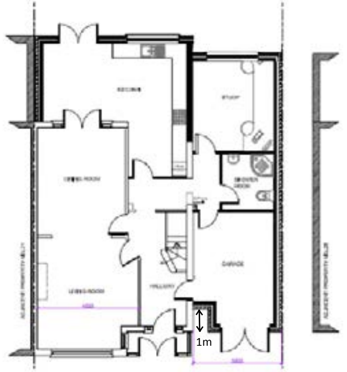
Figure 12: Illustration of a recessed linkage between the garage and the house
