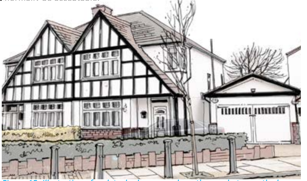
Figure 15: Illustration of a detached garage where the gap between the house is retained
