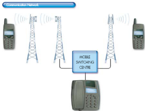
2 The base stations are linked together via dish antenna links or occasionally a land line. Mobile switching centres (telephone exchanges) enable the calls to be transferred to their final destination.
